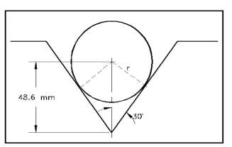
5) Determine the width (x) across the top of the dovetail.
