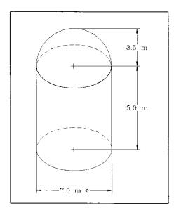
9) Determine the total volume of the tank shown. The top is spherical in shape.
