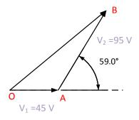
The first phasor has a magnitude of  $V_1$  = 45V (i.e. length of OA) and the second of  $V_2$  = 95V (i.e. length of AB).
